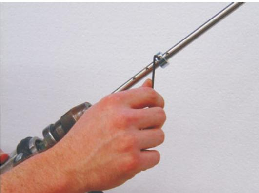
When cutting for the fixation cylinders ZyRillo®, the adjusting ring must be attached with the fixation screw in the existing boot. It does not require the adjusting ring for continuous cutting.
