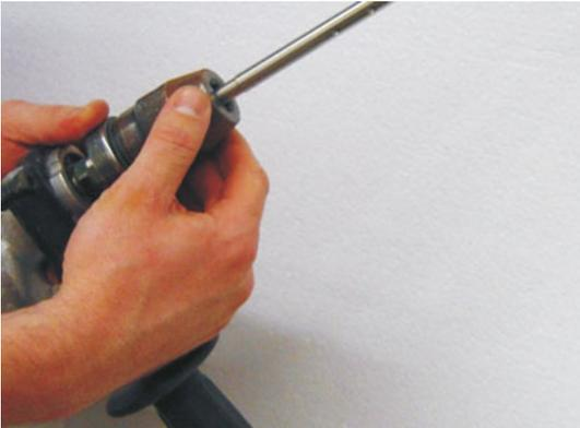
Tension the spindle into the drill chuck.
